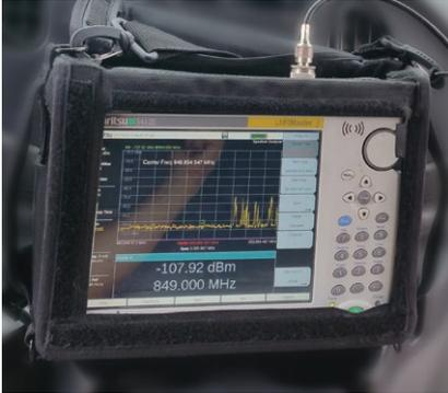
“Starting with the Anritsu S412E System Analyzer and other smart and affordable tools, we were able to build a system that helps customers find and abate interference in just minutes, even in the presence of thousands of signals.”
